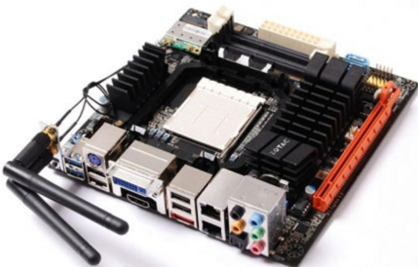
Build the perfect AMD®-powered mini-ITX system with the ZOTAC 890GX-ITX WiFi and AMD® socket AM3 quad, dual or single-core processors. The ZOTAC 890GX-ITX WiFi lets users combine the power of AMD® Phenom™ II, Athlon II™ or Sempron processors with high-performance integrated ATI Radeon™ HD 4290 graphics processing for a perfect blend of CPU and GPU performance in a miniature form factor.
